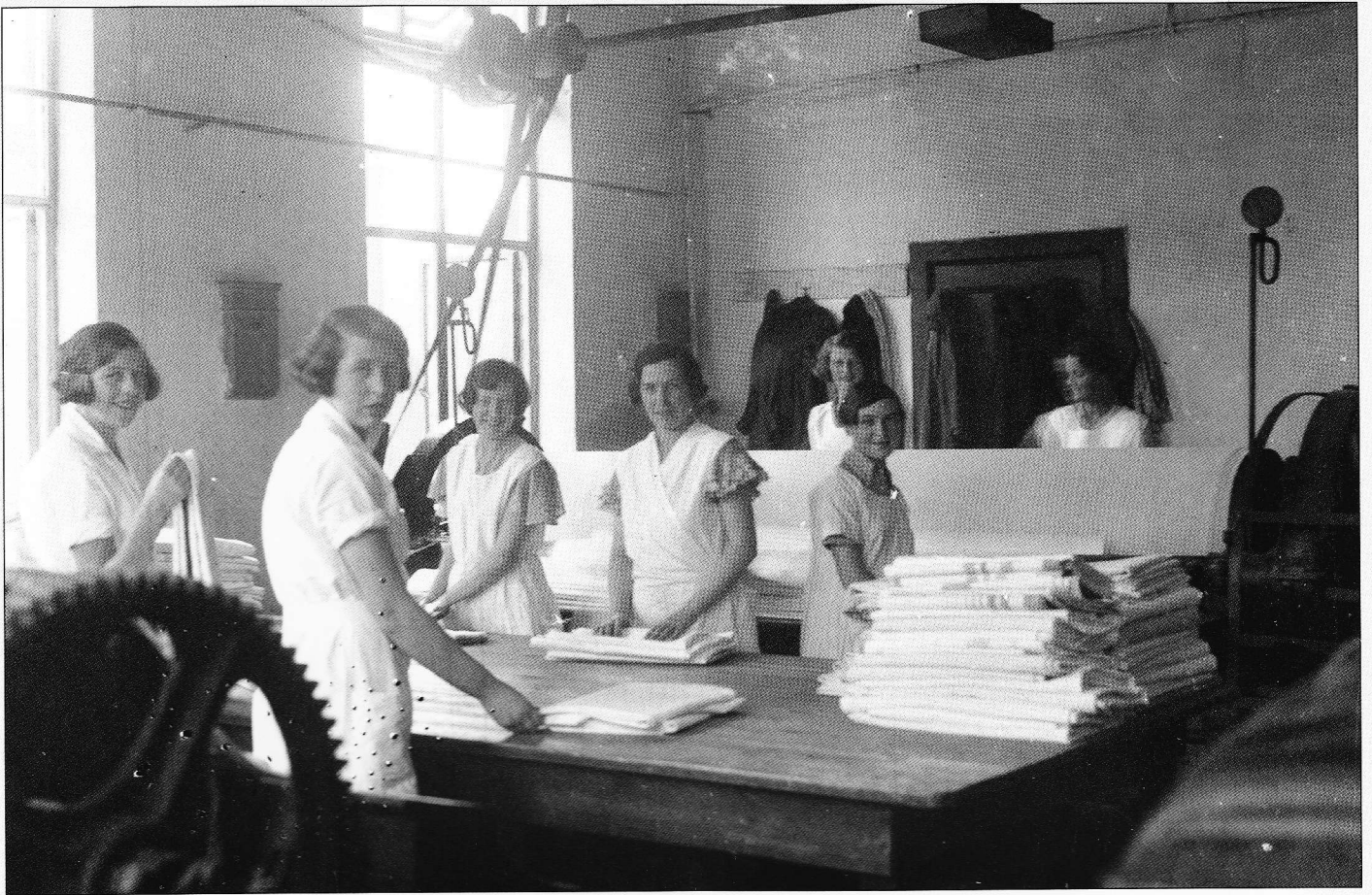
In the 1920s, the shirt industry was one of the most important industries in the City. There were over 40 shirt factories which employed some 8,000 people, mainly women. Most of these factories did their own laundering. After soaping, rinsing and blueing, the shirts were starched and sent to the drying rooms where they were then folded. (FAC 4-14)
